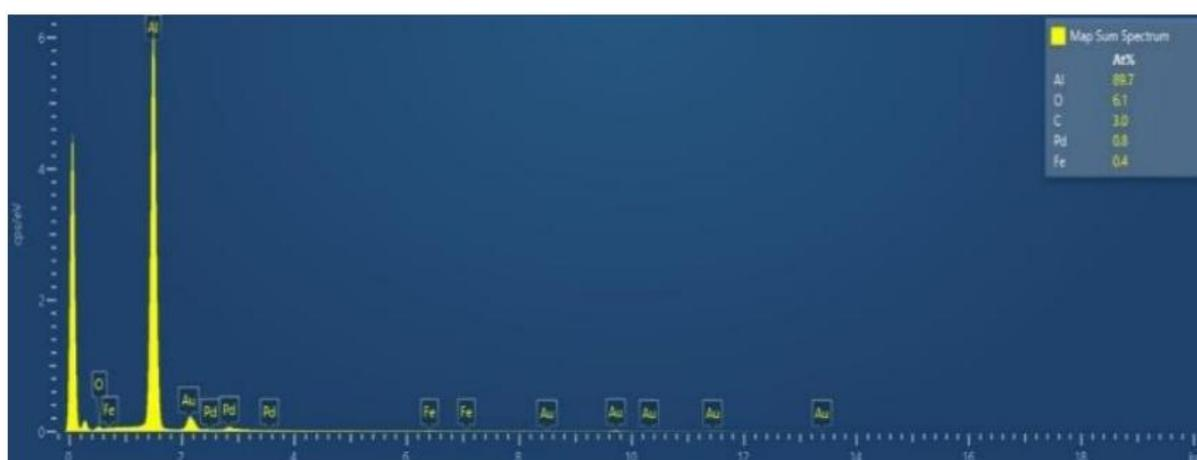
Figure 8: EDS of graphene/Al by ball milling.
